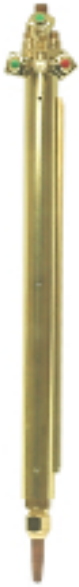
BUG-1274 3-Hose Machine Torch 10" (254 mm) Cutting Torch is the same for Acetylene- Propane-Natural Gas. Only the tip changes.
